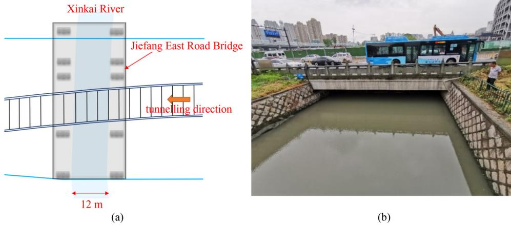
**Fig. 24** Plane position of the new river and the surrounding environment: (a) relationship between the plane position of the new river and the tunnel; (b) surrounding environment of the Xinkai River.
