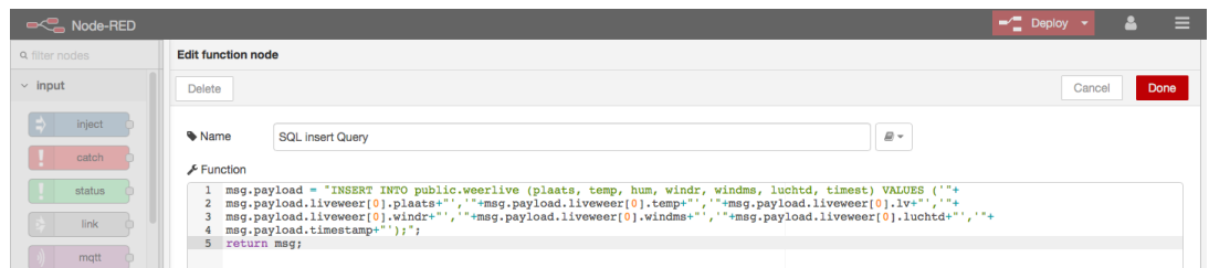
Figure C.5: Settings for the "function" node SQL insert Query
