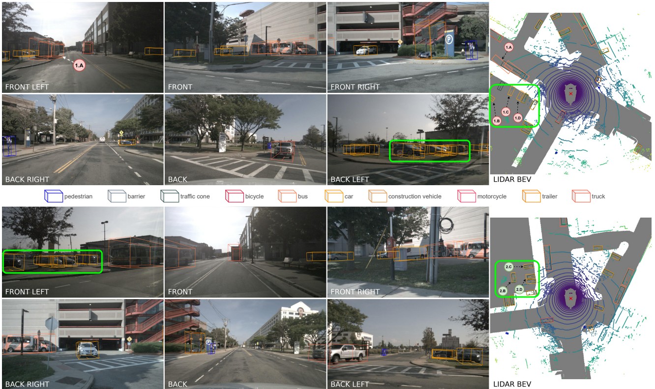
Figure 8. Two consecutive samples from the same scene where the top sample occurs 2 seconds before the bottom sample. We highlight the same region of interest in bright green in both the camera view and the LiDAR BEV for both samples. Best viewed zoomed in.
