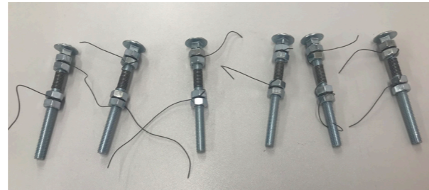
Fig 8.4 Programming SMA wires to become springs with the help of nuts and bolts.
