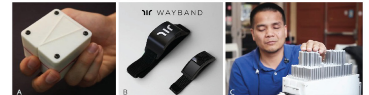
Example devices; A: Animotus-a shape changing haptic interface for navigation [10] B: Wearable haptic navigation device [11] C: Tactile display of on-screen 3d shapes [12]
