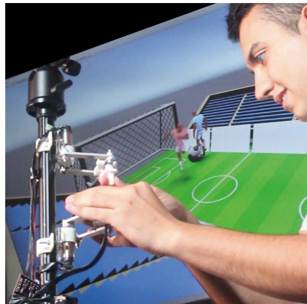
Fig 3.4 DualPanto- force feedback device for tracking movement (Schneider et al., 2018)
