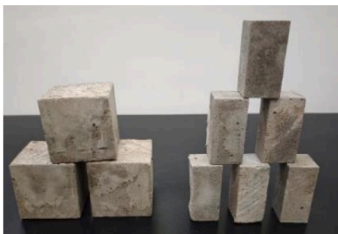
Fig. 1. Cement base specimens after demolding (left) and cut (right).
