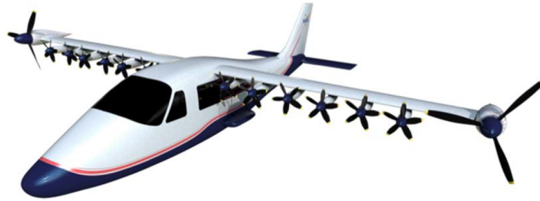
Figure 1.3: The X-57 Maxwell DEP aircraft. (Viken et al. [8])
