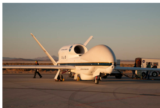
Figure 4.2: Picture of NASA's Global Hawk, with a person standing behind it for size reference 1
