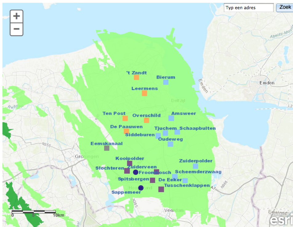
Figure 3.2: Groningen field with 22 production clusters and 4 production regions; orange=Loppersum, blue=Oost, grey=Eemskanaal and purple=Zuidwest. The two blue dots are called 'satellite of production location'; both are 2 production clusters and belong to the purple Zuidwest region, (source: NAM (2017b)).
