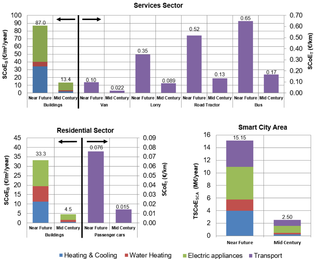
Fig. 8 – Specific Cost of Energy for Buildings (SCoE B in €/m 2 /year) and Transport (SCoE T €/km) per sector (Services sector upper diagram, Residential sector lower left diagram) and Smart City Area Total System Cost of Energy (TSCoE SCA in M€/year) (lower right diagram).
