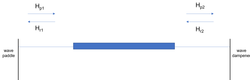
Figure 4.3: Schematic diagram of the four wave signals that are found from the time series measurements by the wave gauges. The arrows show the propagation direction of the wave signal.
