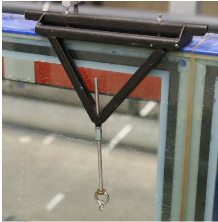
(a) Mooring point attached to basin side.
