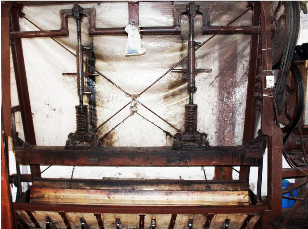
Figure 1 Felting machine. The two arms apply pressure from above while the tank in the bottom whirls the piece around itself. Photography: Aktaş, December 2016, Tire.
