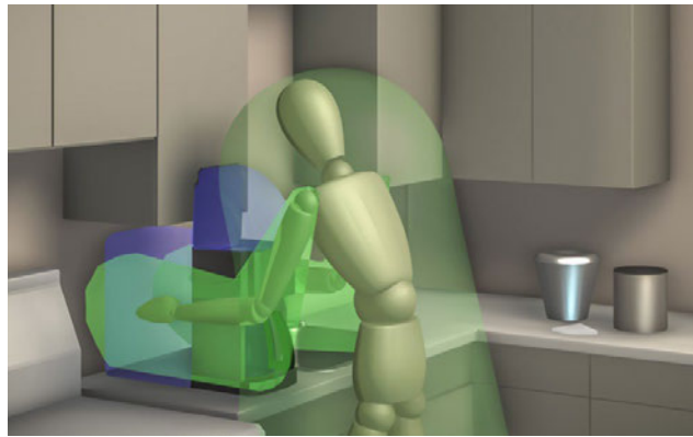
Figure 3 Phantom volume required for the user’s body in relationship to the coffee maker. Note also counter space occupied by the can of fresh coffee, coffee filters, and compost bin.
