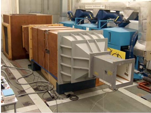
Figure 3.1 Low-speed wind tunnel upstream of the test section and model installation.
