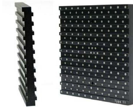
Figure 3.21 Lavisision Type 11 two-level calibration target with dotted grid ( www.lavisision.com ).
