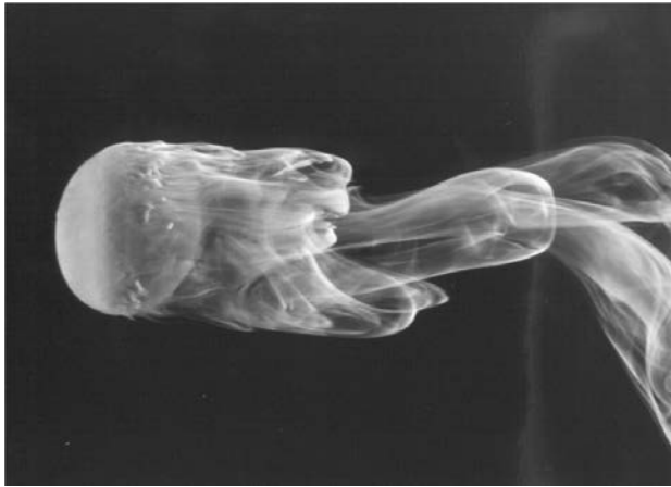
Figure 1.8 Flow visualization of the wake past a sphere at Re_D = 202 . Adapted from Taneda (1956).
