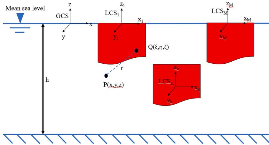
Fig. 1. Definition of the coordinate system for the multiple body interaction problem. *GCS* refers to the global coordinate system and *LCS* refers to the local coordinate system per body.  $Q$  denotes the source point on the immersed body surface and  $P$  denotes the field point anywhere in the fluid domain.
