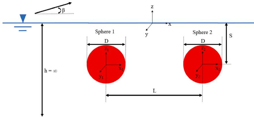
Fig. 5. Two submerged sphere interaction problem (Case 2).
