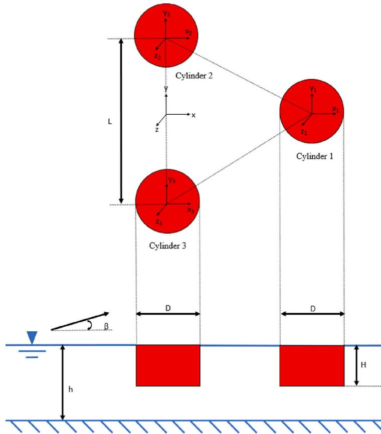
Fig. 10. Three semi-immersed floating cylinders (Case 3).
