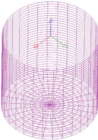
Fig. 3. Cylindrical mesh with 1200 panels used in Case 1.
