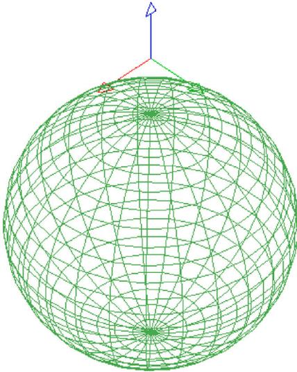
Fig. 6. Spherical mesh with 625 panels used in Case 2.
