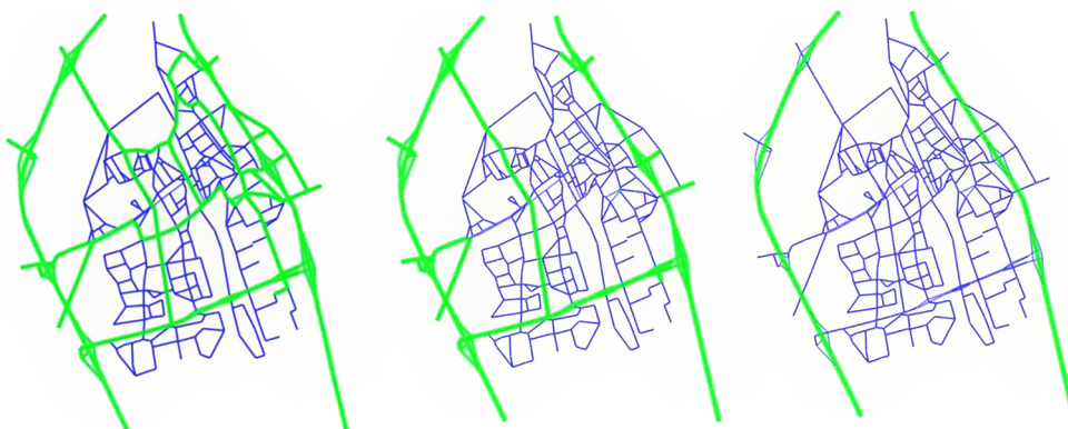
Fig. 1. AD subnetwork variants (from left, respectively): variant 3 (main variant), variant 2, and variant 1 (links that belong to the AD subnetwork are shown with (bright) green and the rest with (dark) blue). (For interpretation of the references to colour in this figure legend, the reader is referred to the web version of this article.)
