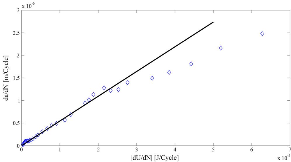
Fig. 7. Correlation between  $da/dN$  and  $dU/dN$  during fatigue delamination.
