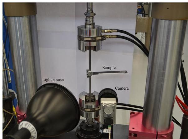
Fig. 1. Fatigue experimental set-up.
