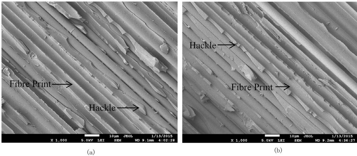
Fig. 9. SEM observations on fatigue fracture surfaces. (a) At a short crack length; (b) At a long crack length.
