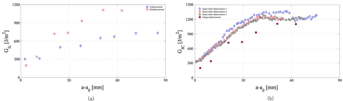
Fig. 3. Comparison of critical resistance increase. (a) Unidirectional vs. Multidirectional; (b) Quasi-static vs. Fatigue.
