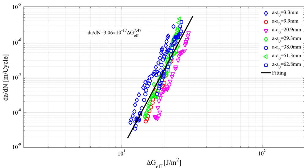
Fig. 5. Fatigue delamination representations via the modified Paris relation.
