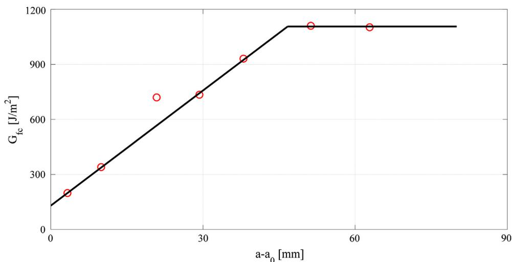
Fig. 2. Interlaminar critical resistance increase with fatigue delamination growth.
