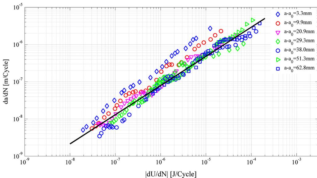
Fig. 8. Energy release in fatigue delamination with different amounts of fibre bridging.
