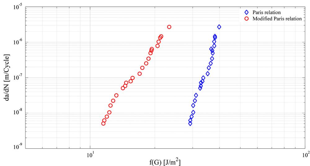
Fig. 6. Data reduction with the Paris and modified Paris relations ( $f(G) = \Delta G$  for the Paris representation and  $f(G) = \Delta G_{eff}$  for the modified Paris representation).
