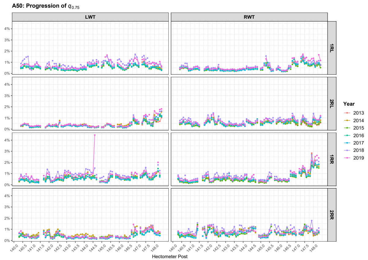
Figure 10.8: q_{0.75} values per year per wheel track and per lane plotted for W = A50 and road sections S_{ij} = 1HRR_j^i for i \in \{1RL, 2RL, 1RR, 2RR\} and 139.9 \leq j \leq 148.4 .
