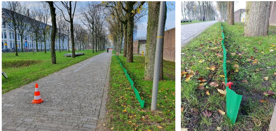
Figure 3.9: Pictures of the plastic barrier used to measure the lateral position (own pictures)
