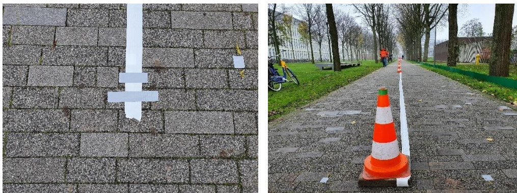
Figure 3.10: Two methods used to attach the white band to the bicycle path (own pictures)
