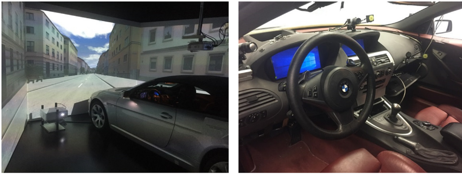
Fig. 1. The TU Munich Driving Simulator. Left: full-vehicle mock-up; Right: cabin.
