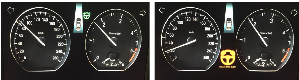
Fig. 3. Photos of the instrument cluster with automation status. Left: automation available, corresponding to Fig. 2b; Right: take-over request, corresponding to Fig. 2e.
