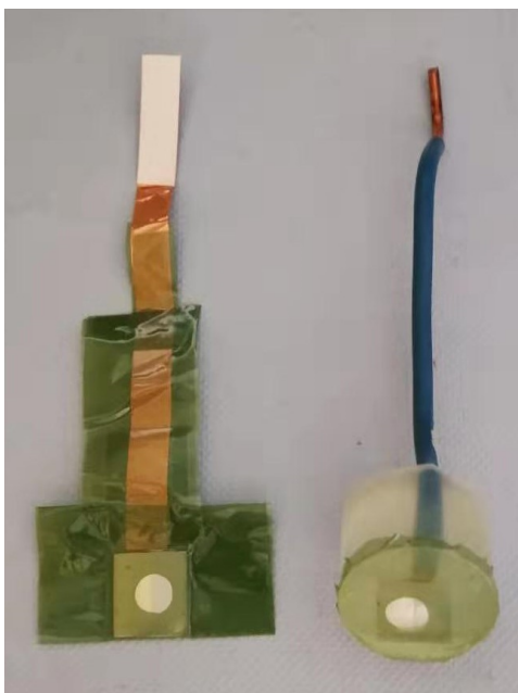
Figure 13: Sample configurations used for LPR measurements.
