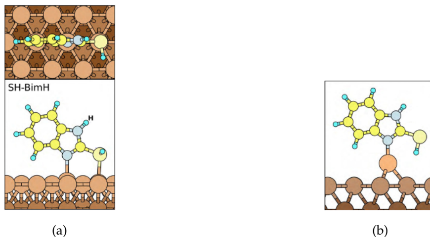
Figure 53: Optimized structures of MBI molecules adsorbed on Cu(1 1 1) (left panels) and the [MBI-Cu ad ] monomer complex (right panels). Color coding of atoms is also indicated: H is cyan, C is yellow, N is sky-blue, and Cu is colored copper-brown with color becoming darker as going from surface toward the bulk. Bond lengths are specified in Åunits. [41]
