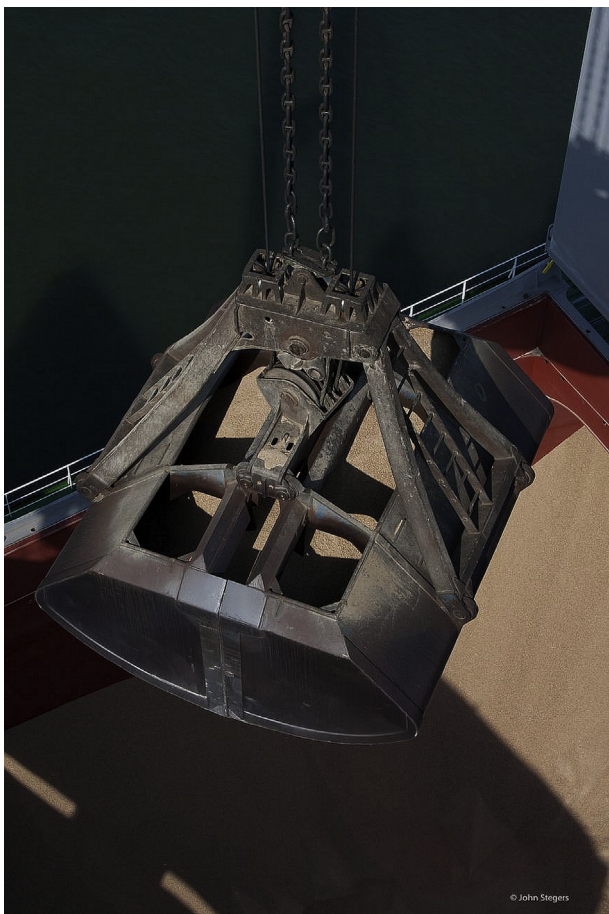
Fig. 10. Closed clam-shell grab used in EBS terminal (Image courtesy of EBS BV).
