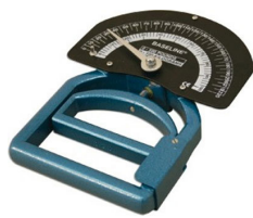
(a) Hand dynamometer using a spring to measure grip force.
