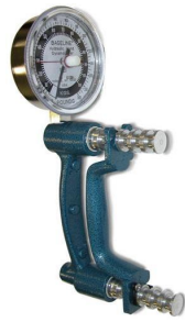
(b) Hand dynamometer using hydraulic pressure to measure grip force.
