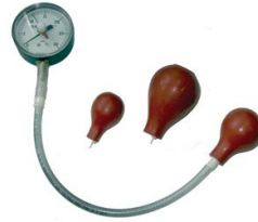
(c) Hand dynamometer using pneumatic pressure to measure grip force.
