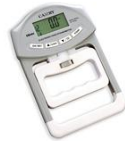
(d) Hand dynamometer using electric strain gauge to measure grip force.
