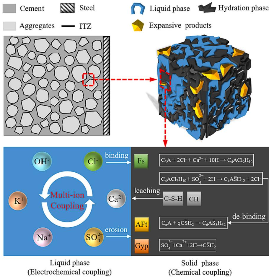
**Fig. 1.** Schematic diagram of mechanisms for concrete under combined chloride-sulfate attack from the perspective of meso-scale modelling, solid-liquid chemical reactions and multi-ion (electrostatic) coupling.
