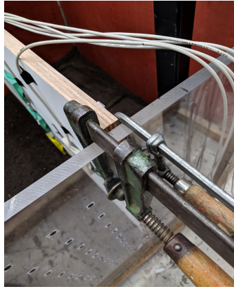
Figure 3.19: Clamps used to restrain the sheetpile during filling.
