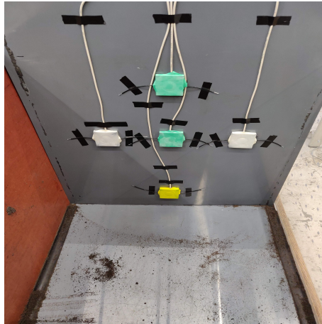
Figure 3.15: PVC sheetpile with sensors attached.
