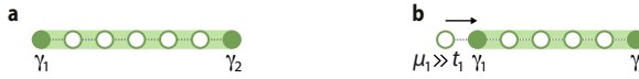
Figure 2.14: Shuttling Majorana modes by acting on the onsite energies. Here, topological Kitaev chain sections with \mu_n = 0 \forall n are depicted with a green background. Unpaired Majorana bound states are indicated with full circles. Setting \mu_1 \gg t_1, \Delta_1 transfers the leftmost unpaired Majorana from the first to the second site. This is a consequence of the perturbation shown in figure 2.5b: as \mu_1 exceeds the inter-dot couplings, the unpaired Majorana is left on the second site.
