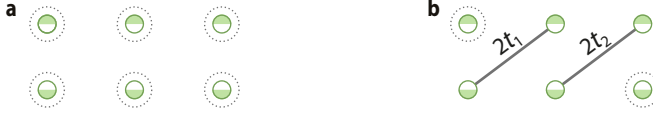
Figure 2.10: a. Three-site Kitaev chain with \mu_n = t_n = \Delta_n = 0 \forall n : there is no protection of the three zero-energy fermions. b. Here t_n = \Delta_n \neq 0 \forall n . There is one protected fermion localized in sites 1 and 3.
