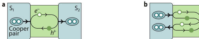
Figure 2.27: Illustrations of a . Supercurrent carried by an ABS via resonant Andreev reflection b . An ABS formed in a (semi-)conductor coupled to a single superconductor.
