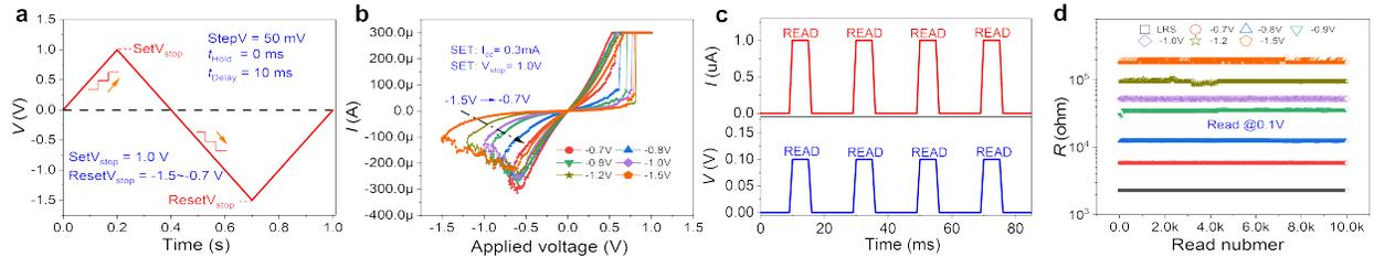
Fig. 3: a) Linear Sweep Voltammetry (LSV) operation for I-V measurement. b) I-V curves obtained by the method in a), where compliance current is 300 uA and RESET stopping voltages vary from -1.5 to -0.7V. c) READ operations for specific resistance states. d) Seven of the Read-number-dependent resistance states obtained by the method in c)
