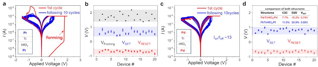
Fig. 2: a) I-V curves of traditional ReRAM devices with an electroforming process. b) Device-to-device (D2D) variation of 20 devices from the same structure as the one in a). c) I-V curves of Pd-based ReRAM devices without an electro-forming process. d) D2D variation of 20 devices from the same structure as the one in c). The inset table is a comparison in cycle-to-cycle (C2C) variation, D2D and V<sub>SET</sub> for both structures.
