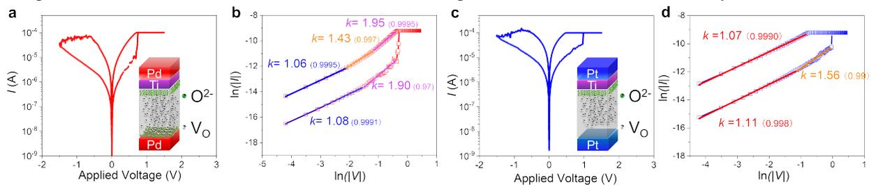
Fig. 4: a) The I-V curve of Pd/HfO<sub>2</sub>/Ti/Pd to be fitted. b) Double-logarithm fitted plot from positive bias of a). c) The I-V curve of Pt/HfO<sub>2</sub>/Ti/Pt to be fitted. d) Double-logarithm fitted plot from positive bias of c). The inset diagrams in a) and c) show schematics of corresponding structures, where they emphasize the interface of PdO<sub>x</sub>/HfO<sub>2-x</sub>.
