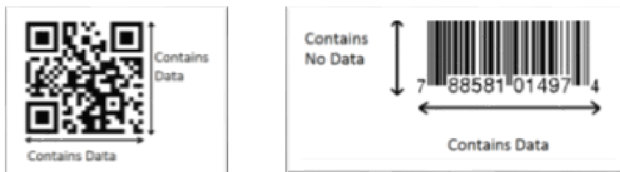
Figure 8: QR code vs. One-dimensional barcode (Kieseberg et al., 2010)
