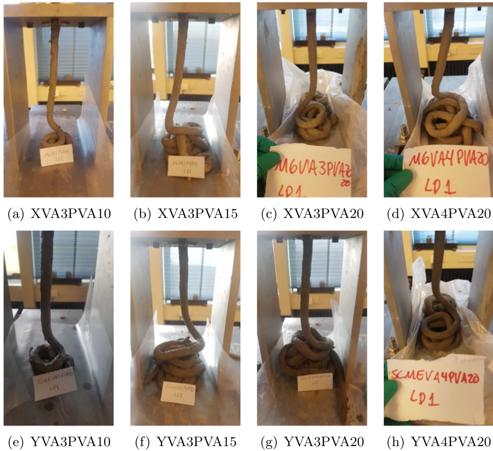
Fig. 13. Visual inspection of extruded material for different levels of PVA fibre reinforcement.
