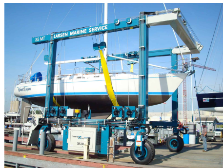
(b) Example of a travel lift (Kendrick Equipment, 2023)
