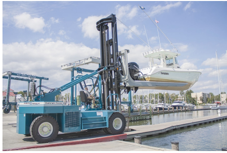
(a) Putting the vessel in the water with the forklift (Marine Travelift, n.d.)
