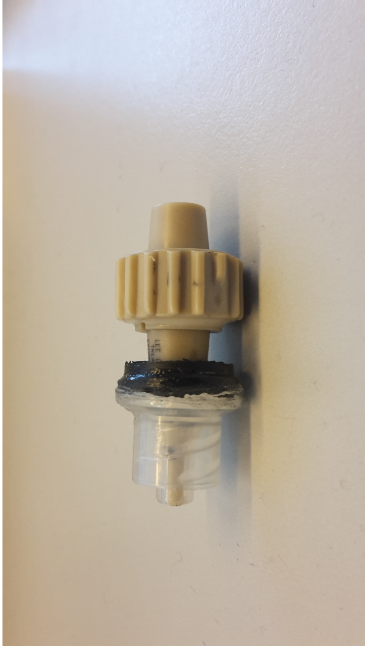
Figure 4.5: Makeshift adapter used for cold testing.
