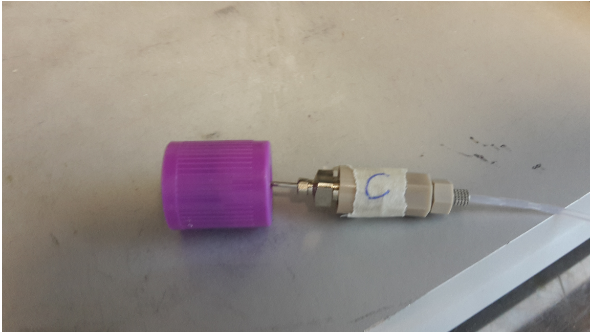
Figure 5.1: The metal needle is blocked by the rubber test tube cap, to perform a leak test. The tubing leads to the pressure/temperature block which in turn leads to a solenoid valve which allows/disallows propellant to pass through.
