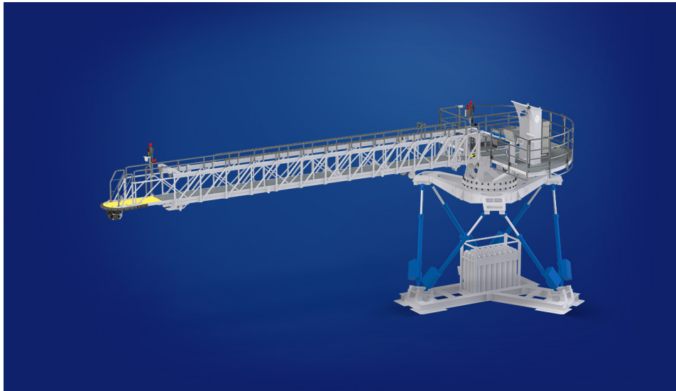
Figure 2.9: An example of a motion compensating platform 'The Ampelmann' used to safely transfer personnel from a vessel to an offshore structure. The platform is able to compensate for all 6 degrees of freedom of the vessel, meaning the platform does not move during transfer [3].
