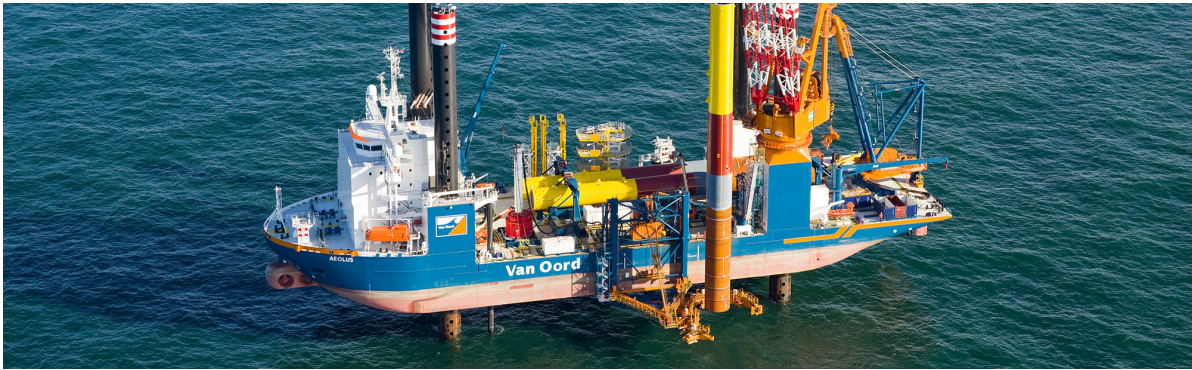
Figure 1.3: A jack-up vessel upending a monopile. Note the gripper frame at the side of the vessel. 1
