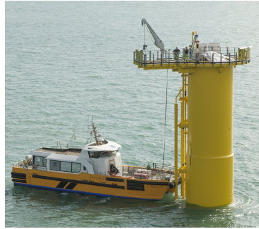
Figure 1-2: Windcat 10 at monopile. [2]
