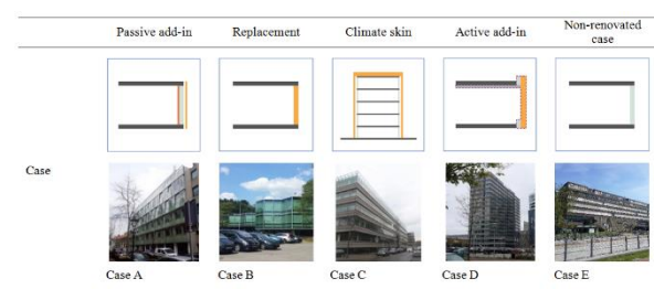
Figure 1: Different scale of façade renovation strategies
