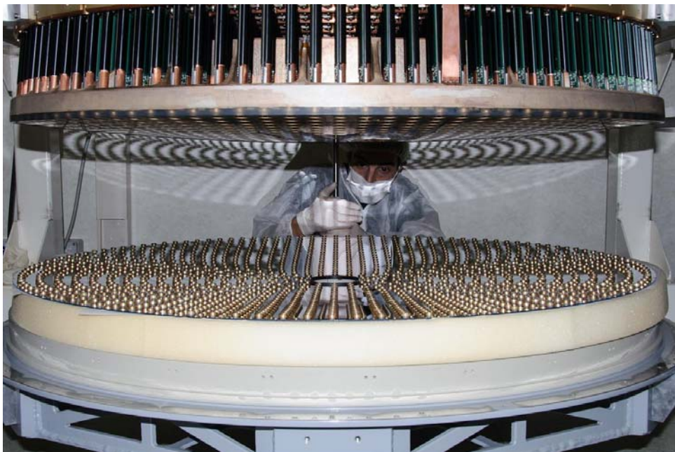
Figure 5.8: A secondary deformable mirror (1.2 m diameter) developed using 1170 voice coil actuators that have a stroke of 100 \mu\text{m} with local positioning control (source [13])
