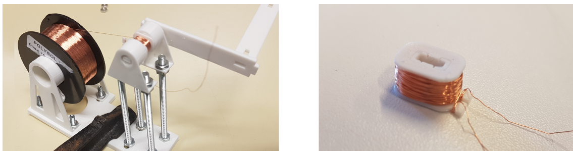
Figure 4.62: Left: Manual coil winding assembly. Right: Wounded coil
