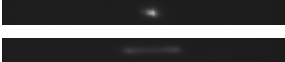
Figure 5.3: Top: stationary beam reflected from the original scanner. Bottom: moving beam reflected from the original scanner at max amplitude
