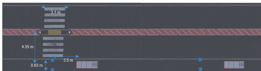
Fig. 2. A bird's eye view of the road, developed using Unity, illustrating the pedestrian crossing location: with zebra crossing (left two blue crosses) and without zebra crossing (right two blue crosses). The bottom cross was used to align the standing position for all pedestrians, who were hidden behind an obstacle (e.g., bus stop), which is depicted as the grey block on the right hand of each crossing location. These were used to ensure pedestrians and drivers were concealed from each other prior to an interaction (not all bus stops had a concealed pedestrian). Pedestrians stepped out to the top cross when they heard a beep, signifying the start of a crossing trial, and stopped at the pedestrian refuge (the yellow block in the middle of the street), before returning to the blue crossed as the end of the trial. (For interpretation of the references to colour in this figure legend, the reader is referred to the web version of this article.)
