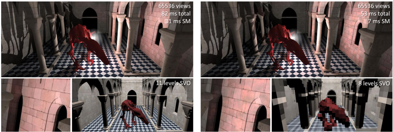
Figure 13: Effect of hierarchy resolution in the Sibenik scene. While the shadow map rendering cost is significantly reduced, using a too low hierarchy resolution causes inaccurate shadow maps, resulting in missed or exaggerated occlusions and artefacts.
