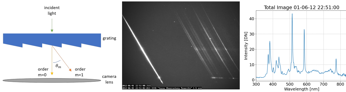
FIGURE 2: Left: Schematic of a transmission grating which lets the first-order spectrum through. Middle: Event 01-06-2012, 22:51:00; zeroth-order meteor (left of the image) and its first-order spectrum (right of the image) seen from CILBO observatory, in Tenerife. Right: Intensity of the first-order spectrum in digital numbers, after the spectrum was retrieved from the total image in the middle .
