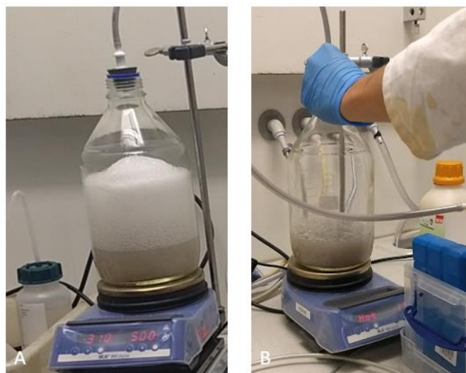
Figure 47 Before(A) and after(B) addition of anti-foaming agent. The foam in picture A would rise even higher and end up in the acid trap if the system was not shut down in time.
