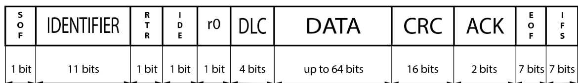
Figure 6.2: A standard CAN message structure: 11-Bit Identifier [22]
