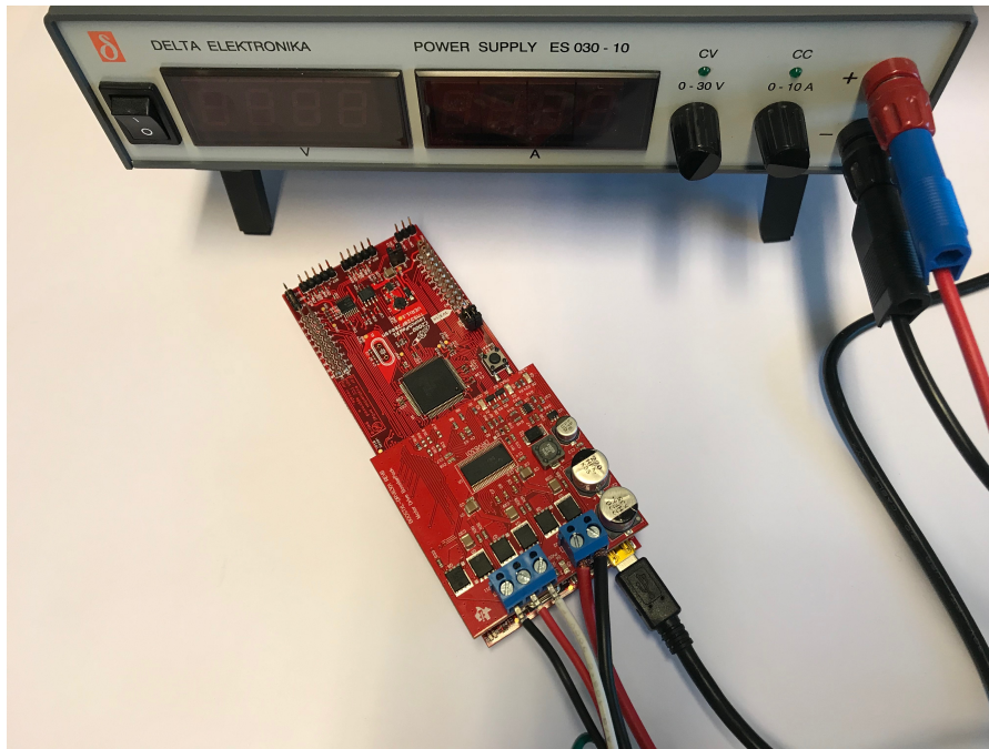
Figure A.38: The LaunchPad/BoosterPack combo with everything connected.
