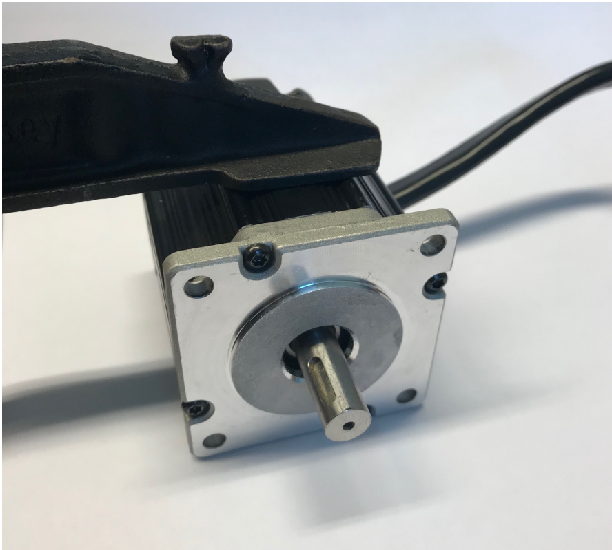
Figure A.39: Make sure the motor is clamped to the table firmly.
