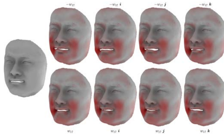
Figure 7.28: Visualization of QSPLOCS using random initialization: The 17th quaternion sparse component on the “face” motion capture from [66]. Models corresponding to -w_{17} (top) and w_{17} (bottom) along the four dimensions of the 17th component are displayed. Color coding shows the magnitude of vertex displacements inside the components.
