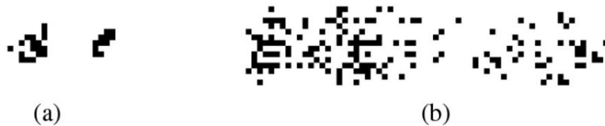
Figure 2.16: Examples of a small cluster of bit upsets (a) and a burst event characterized by several single bit upsets following a rectangular geometrical shape (b). Figure was taken from [58].
