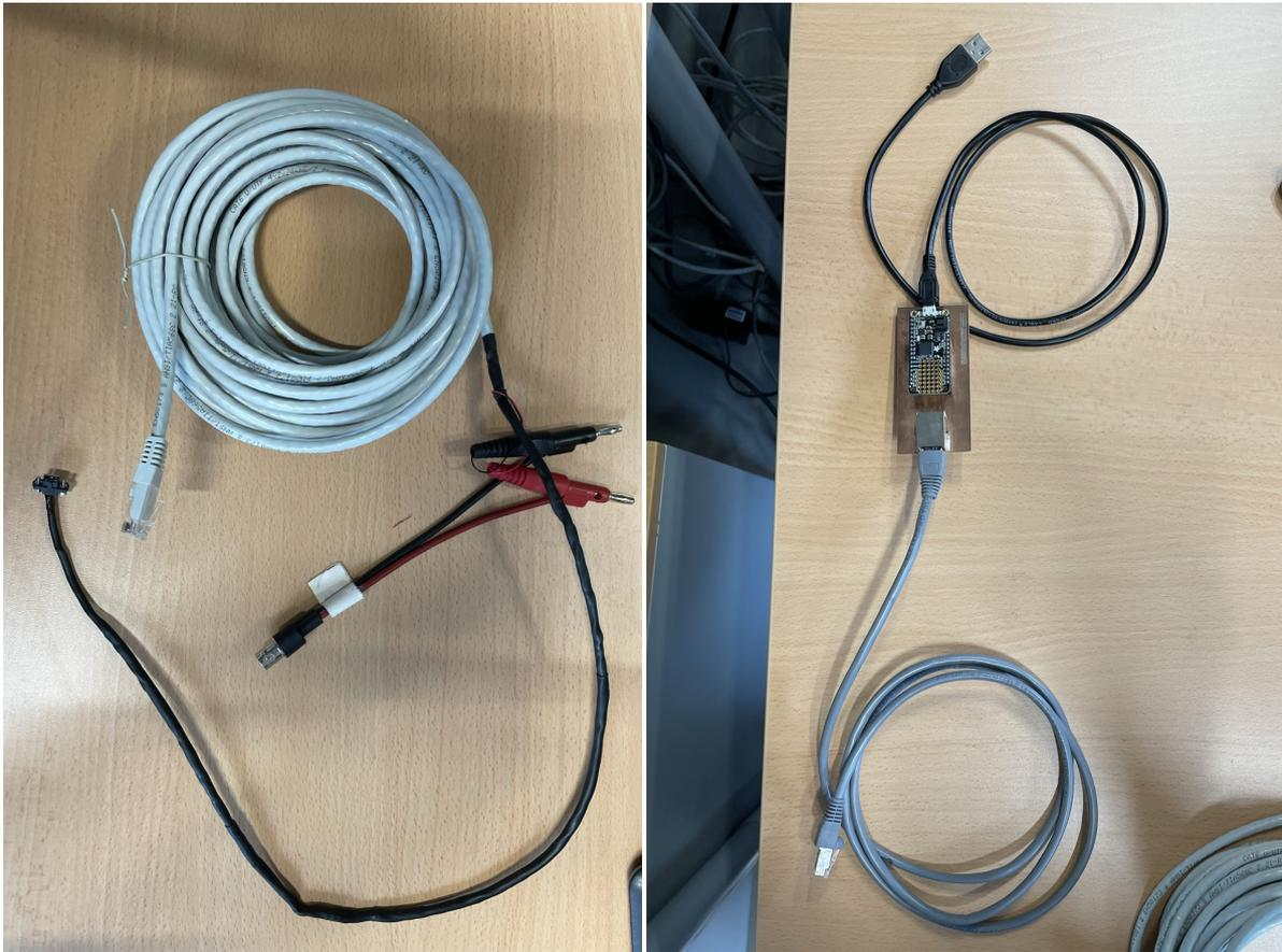
(a) Cable made for from the payload to the patch panel.
