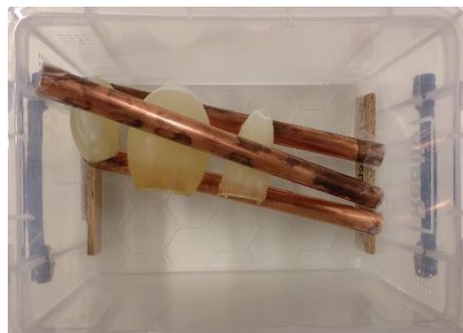
Figure 11. Phantom using \text{Al}_2\text{O}_3 as scattering particles before being filled with the parenchyma tissue mixture.
