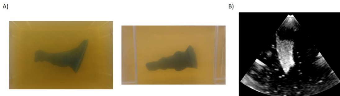
Figure 21. Phantom used for the development of an automatic or semi-automatic segmentation algorithm. It consisted of a dinosaur shape made of PVA with aluminium oxide particles as inclusion in a gelatin mixture. A) Photo of the phantom. B) US image of the phantom.
