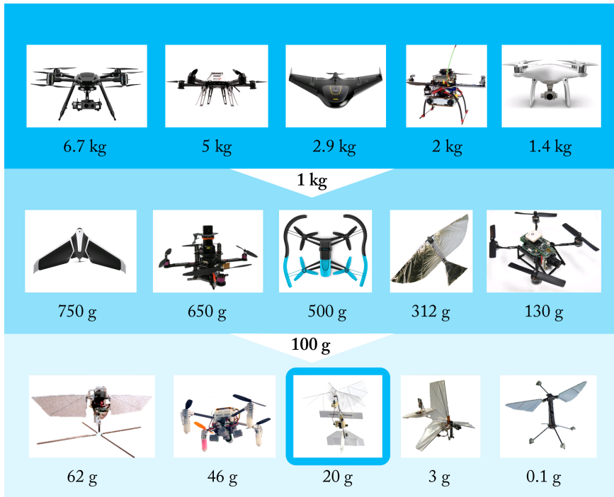
Figure 1.1: The weight spectrum of Micro Air Vehicles; from kilograms to sub-grams. The examples show the variety in types of platforms, and also indicate what types are common for each weight class. The 20 g DelFly Explorer, which is developed in this thesis, is indicated on the bottom row. 6.7 kg Altura Zenith ATX8 [7]. 5 kg AscTec Neo [8]. 2.9 kg UX5 HP [9]. 2 kg PIXHAWK [10]. 1.4 kg Phantom 4 [11]. 750 g DISCO FPV [12]. 650 g AscTec Pelican [13]. 500 g Bebop 2 [14]. 312 g Robo Raven [15]. 130 g Nano+ [16]. 62 g Robotic Hummingbird [17]. 46 g Ladybird V2 [18]. 20 g DelFly Explorer (this thesis). 3 g DelFly Micro [19]. 0.1 g Robobee [1].
