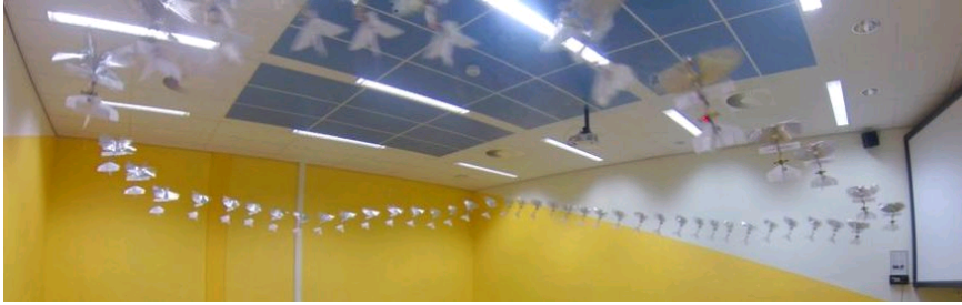
Figure 1.4: Time lapse image showing the DelFly Explorer autonomously exploring a room by using its onboard stereo vision system for obstacle avoidance.
