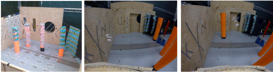
Figure 4.17: Left: Test room of 6×6 meters where flight tests have been performed. The room contains four poles of 40 cm diameter that form obstacles. The locations of these obstacles were different for each test flight. Middle and Right: Images of two setups to test the robustness of the system to poorly textured obstacles. The orange poles do not have additional texture. Middle: room with two walls, enclosed by the orange poles. Right: same room as in the left case, one pole is placed inside the enclosed area.
