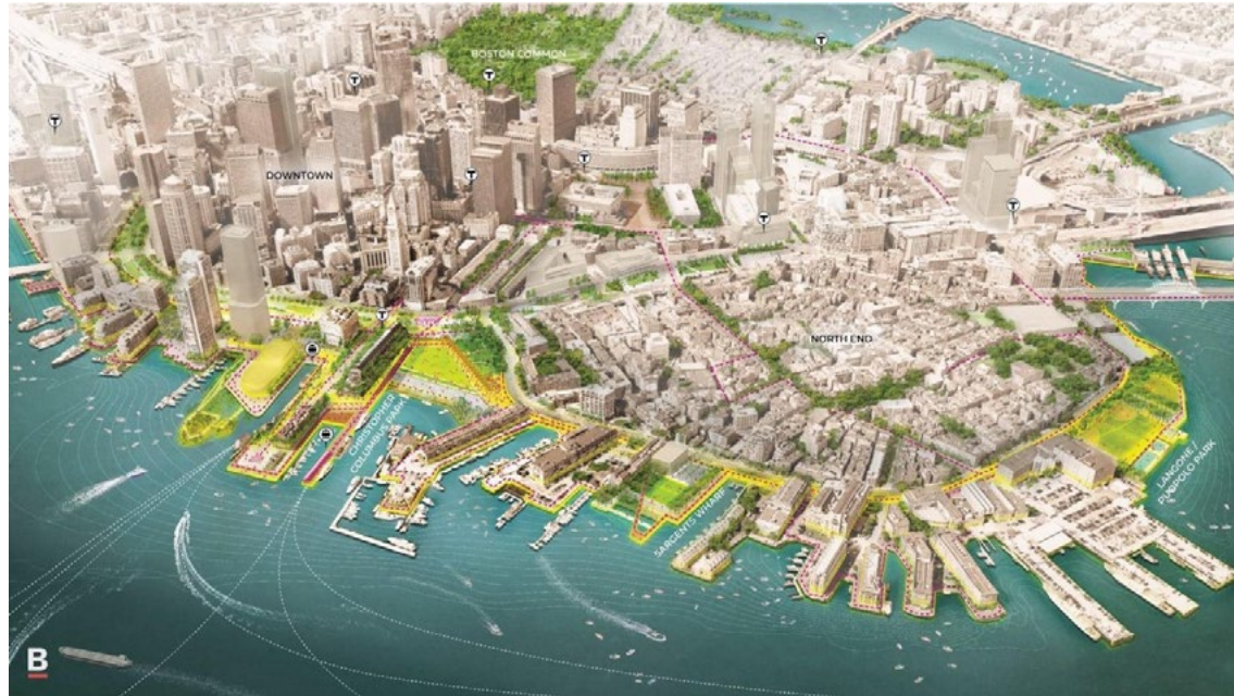
Figure 1 The Downtown section of the Resilient Boston Harbor Vision shows a green park around the coastal edge of the city with a component of a flood protection barrier (visualization from the City of Boston, by Landscape Architecture firm SCAPE).
