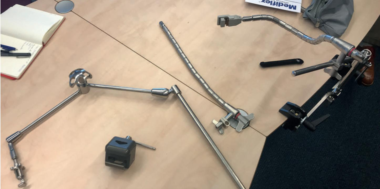
Fig 3.30. **Surgical mechanical arms.** Martins arm on the left and Flexible arm in the right.
