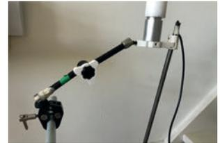
Fig 9.4. **Simple test whereby mount is clamped on 15 mm bar holding a weight of 2 kg.**
