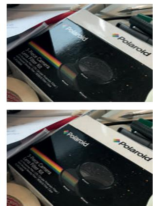
Fig 3.20. Test with polarisation filter. A: without polarisation filter. B: with polarisation filter. Still the amount of glare is heavily subjected to slope.
