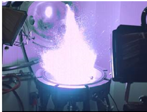
Figure 9: Visualization of the fireball and hot particles generated by a 5-kJ pyrotechnical igniter in the open Fike 20-l sphere (0.34 m in diameter)
