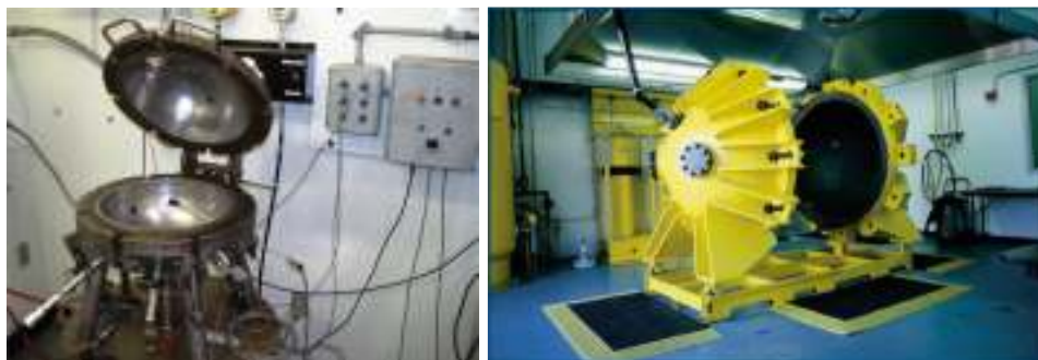
Figure 1: Photo of 20-l sphere (left) and 1-m 3 chamber (right) operated by Fike Corporation
