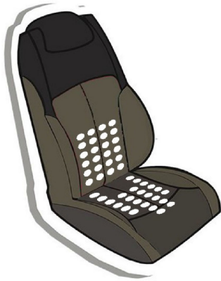
Fig. 3. Illustration of the vibrotactile seat and the location of the 48 vibration motors (i.e., white circles). The motors are arranged in two matrices of 6 \times 4 motors (one matrix in the seat back, and the other matrix in the seat bottom).
