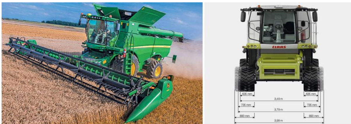
Figure A.1: John Deere S790 combine and 635F platform (left). Width dimensions for the Lexion 780, 770 and 670 (780 being the largest) (right).
