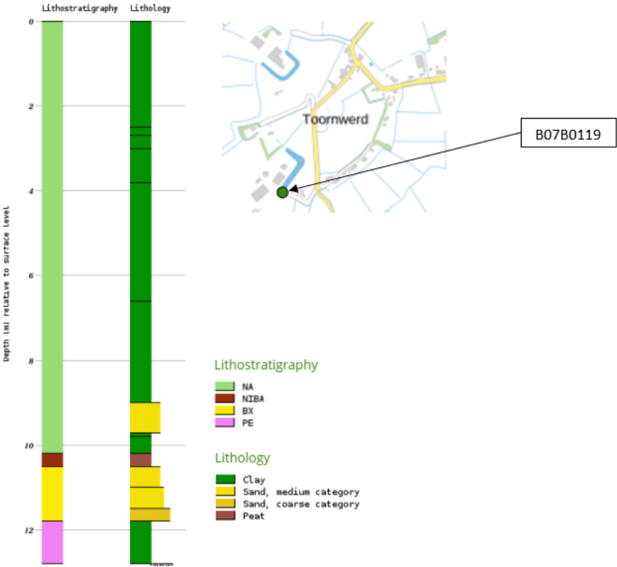
Figure 16: DINOloket borehole data for Toornwerd.
