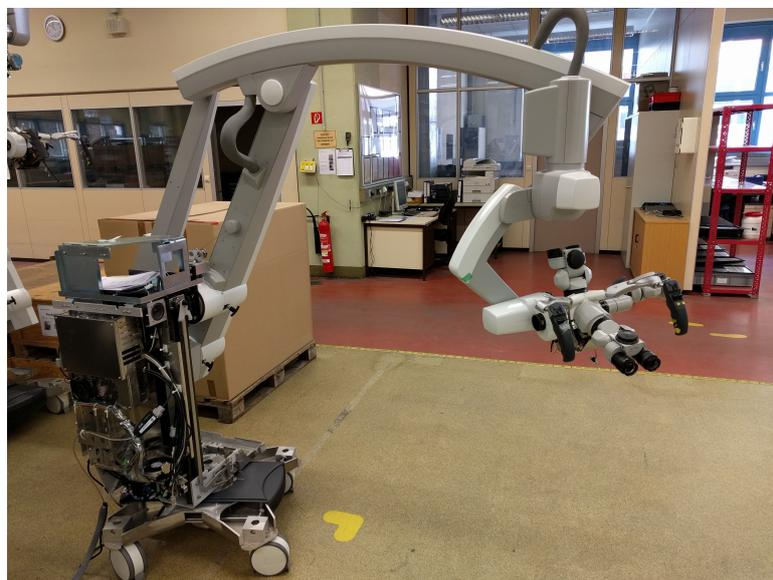
Figure 7.4: Double balancing system subjected to measurements.
