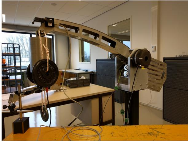
Figure 3.2: Test set-up for the Arm module. Stand for the sensor in lower left corner.
