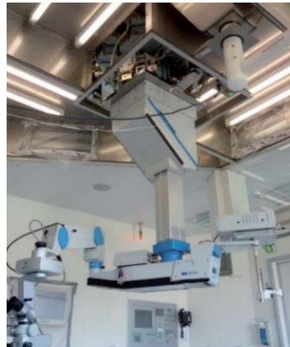
(c) Microscope mounted to the Hummingbird vibration isolation platform [12].
