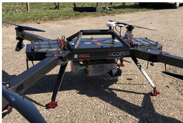
Fig. 2. RICOPTER platform equipped with Riegl VUX-1LR scanner and two oblique Sony Alpha 6000 cameras used for capturing H3D.
