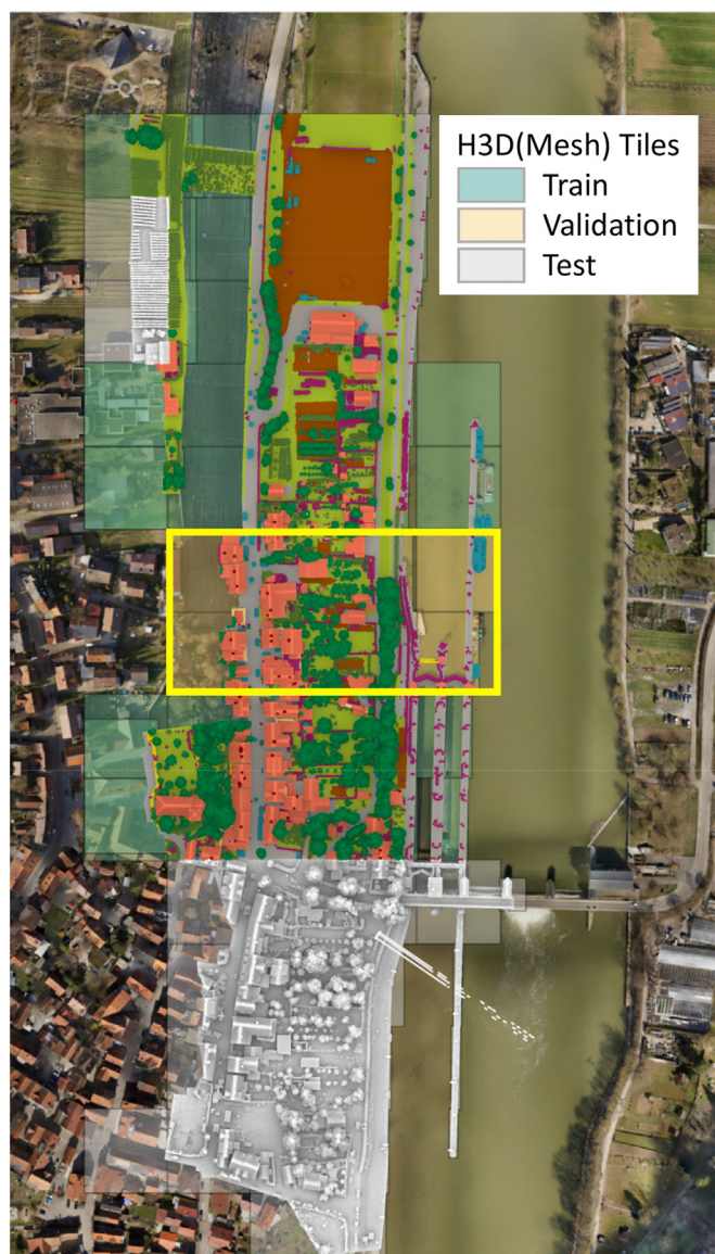
Fig. 1. Overview of H3D(PC) and H3D(Mesh) using an orthophoto basemap. H3D(PC) is partitioned into training set (indicated by class colors ; see Table 1), validation set (indicated by class colors and marked by a yellow box ), and test set ( grey ). H3D(Mesh) is organized in tiles that exceed the annotated point cloud (see Section 2.5). The data splits of H3D(Mesh) are partitioned in accordance with the respective H3D(PC) splits. They are shown in semi-transparent manner (see legend).
